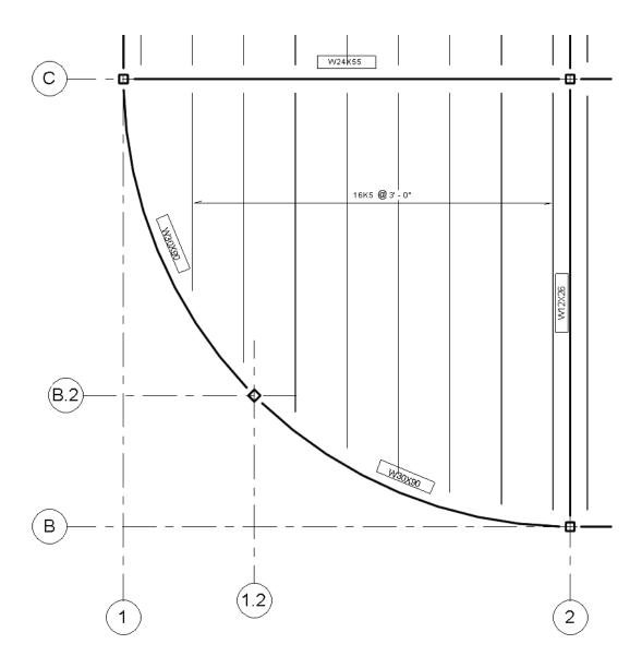
Figure 4.1-12 Structural Beam System with tag added
