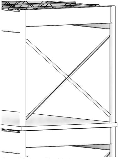
Figure 4.1-10 Structural (cross) bracing
