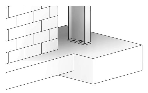
Figure 4.3-3 Wall foundation joined to isolated foundation
