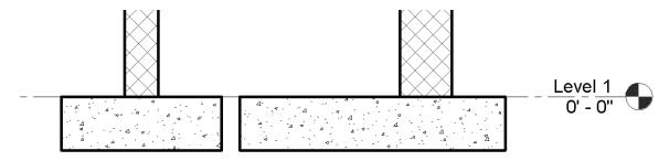
Figure 4.3-6 Wall foundations; Bearing (left) and Retaining (right)
