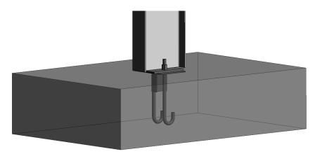
Figure 4.3-1 Isolated foundation added at structural column
