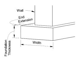
Figure 4.3-4 Wall foundation (bearing) dimensions
