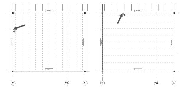
Figure 4.1-11 Defining Structural Beam System direction; hover cursor over beam
