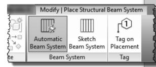
**Tag on Placement** allows the new brace to automatically be tagged in the current view.
