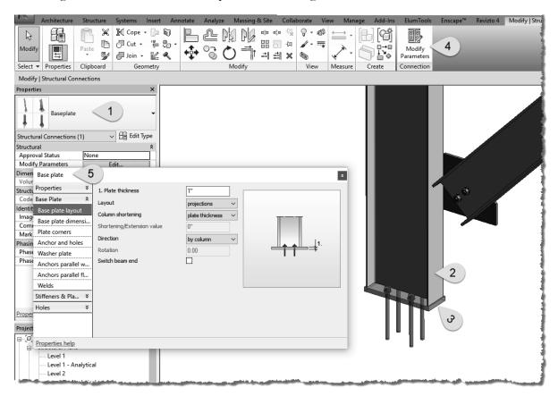
Figure 4.2-1 Structural Connections workflow
