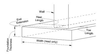
**Figure 4.3-5** Wall foundation (retaining) dimensions
