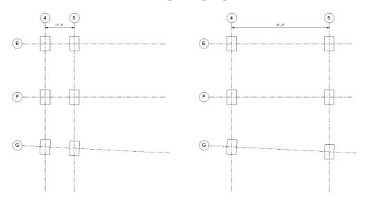
Figure 4.3-2 Isolated foundations added at grid intersections update automatically
