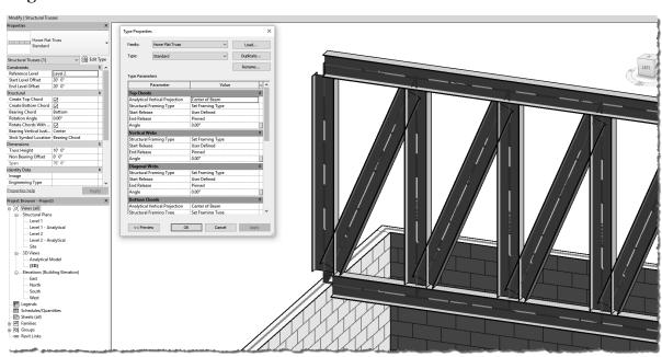
Figure 4.1-8 Structural truss and its properties
