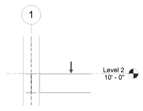
Figure 4.1-1 Structural beam default vertical alignment
