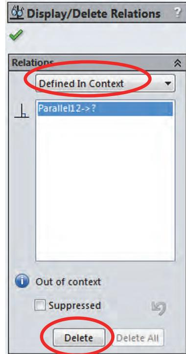
**96.** – After deleting this relation, our sketch is still in an undesired state, we have both unsolvable and over defined geometry, as we can see in the status bar and by the red and brown geometry.
