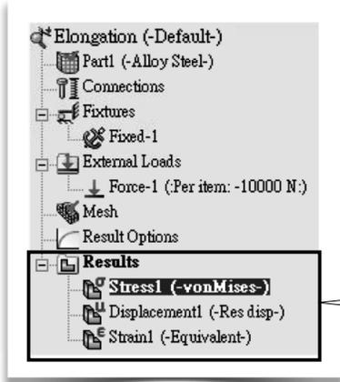
[2] As mentioned earlier (1.1-7), by default, results for **Von Mises Stress, Resultant Displacement, and Equivalent Strain** are created. Note that **Stress1** is highlighted, meaning it is active and displayed in the **Graphics Area**.
