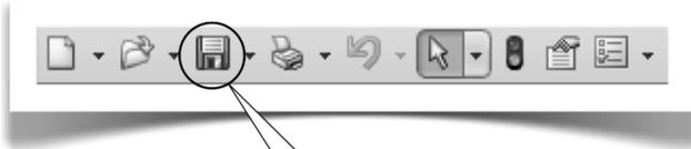
[1] Click **Save** to save the document with the name **Cantilever**. Two files are created in your working folder: **Cantilever.SLDPRT** and **Cantilever-Elongation.CWR**; the former is the main project file, while the later stores the result data generated by a finite element solver. Other files, if any, are not relevant; they can be deleted.
