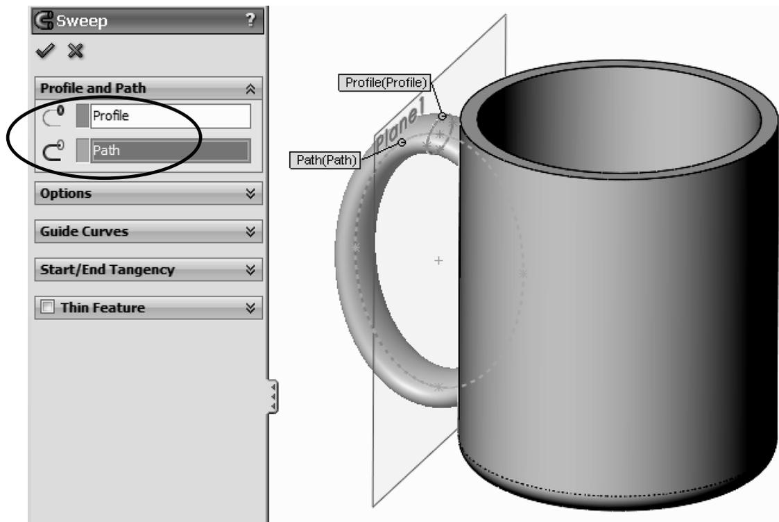
**155.** - Notice the sweep is also inside the cup. We will make a cut to fix this. Create a sketch in the flat face at the top of the cup. Select the inside edge at the top and use “**Convert Entities**” from the Sketch tab to convert the edge to sketch geometry. Select the “**Extruded Cut**” icon and use the option “Up to next” from the end condition drop down selection.
