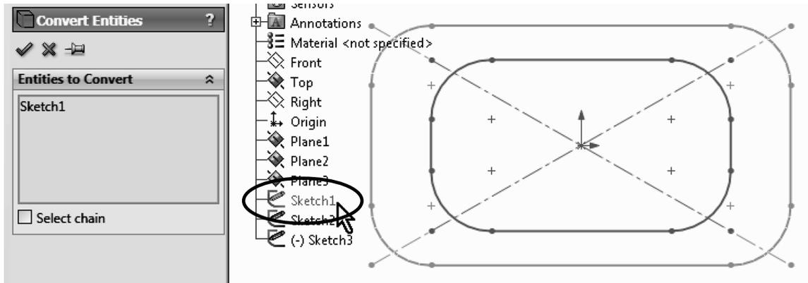
177. - For the last profile select 'Plane3' from the FeatureManager and create a new sketch. Draw a circle and add a geometric relation to make it “Tangent” to the horizontal line in *Sketch2* as indicated by the arrows. This relation will fully define the sketch. Exit the sketch to finish.
