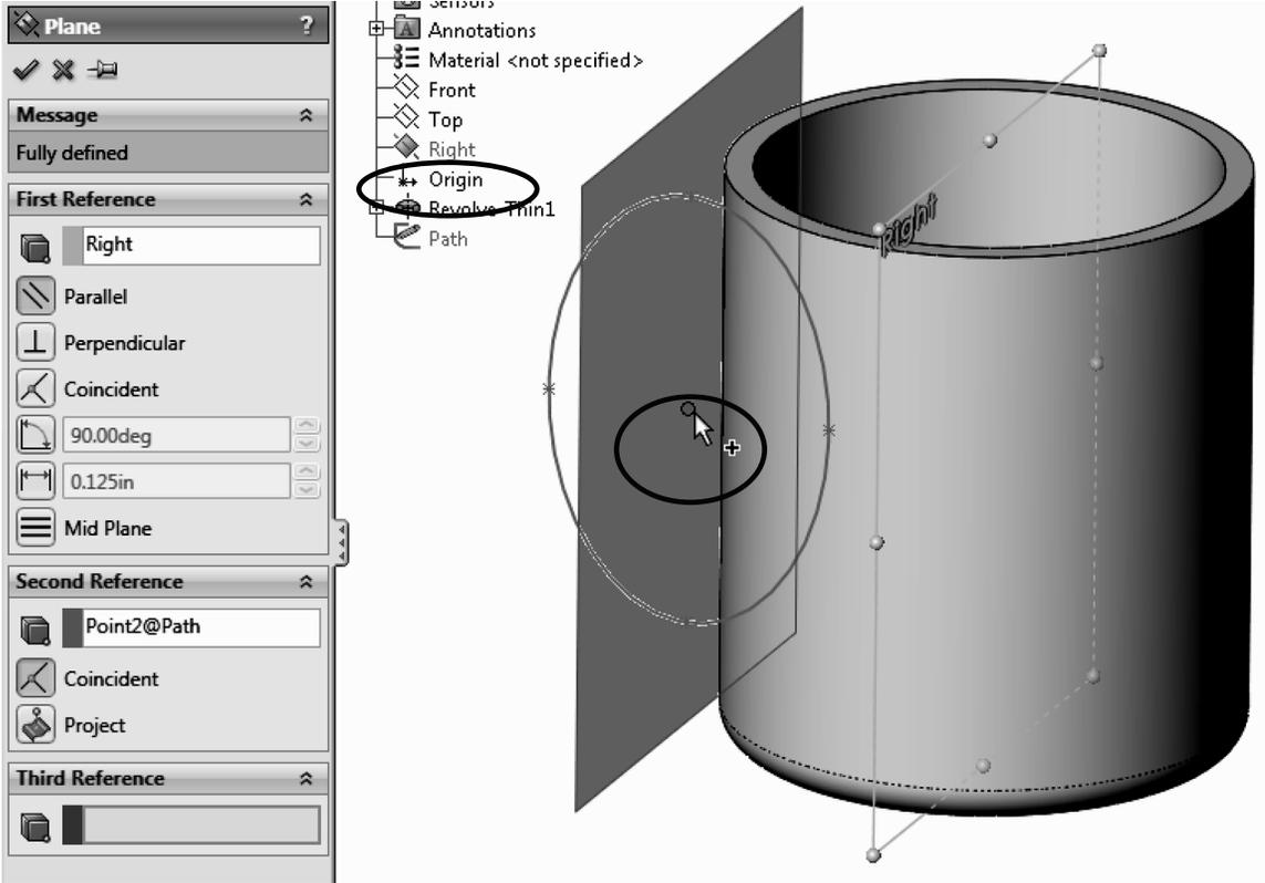
**153.** - Select the plane just created and draw the next sketch. Start the center of the ellipse at the top point of the previous sketch's ellipse. Add a coincident relation if needed. Remember to add a horizontal relation between the points of the major (or vertical to the minor) axis. Exit the sketch and rename it '*Profile*'.
