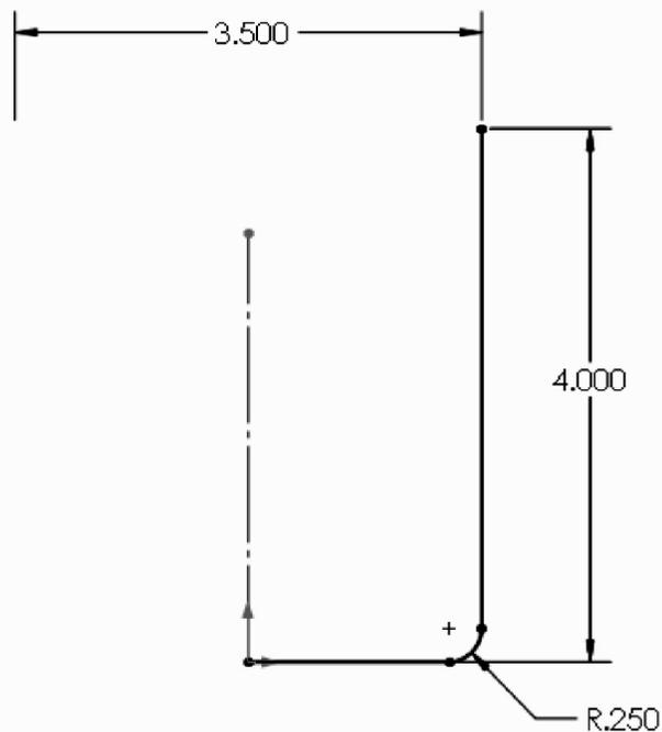
150. - After selecting the “**Revolve Boss/Base**” command we get a warning telling us about the sketch being open. Since we want a thin revolved feature, select “No”.
