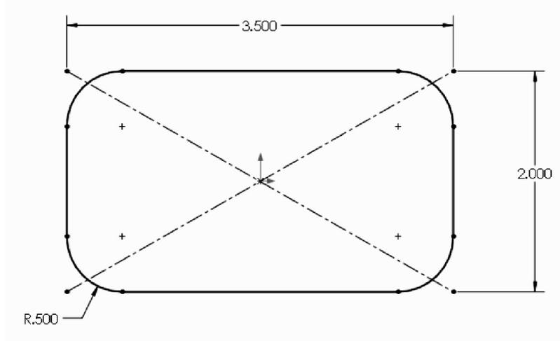
**175.** - Still in the Top view, select 'Plane1' from the FeatureManager and create the second sketch. Use the “**Center Rectangle**” tool; be sure to start in the origin and make the rectangle's corner coincident to the previous sketch's diagonal line. Add a 2.5” width dimension and the 0.5” “**Sketch Fillet**” to fully define the sketch. Exit the second sketch when finished.
