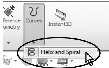
166. - In the Helix/Spiral command select “Pitch and Revolution” from the “Defined by:” selection box and “Variable Pitch” in the Parameters box. After selecting it we are presented with a table to fill in the values for the Helix. Fill in the following values. Notice the helix preview. Click OK when finished.
