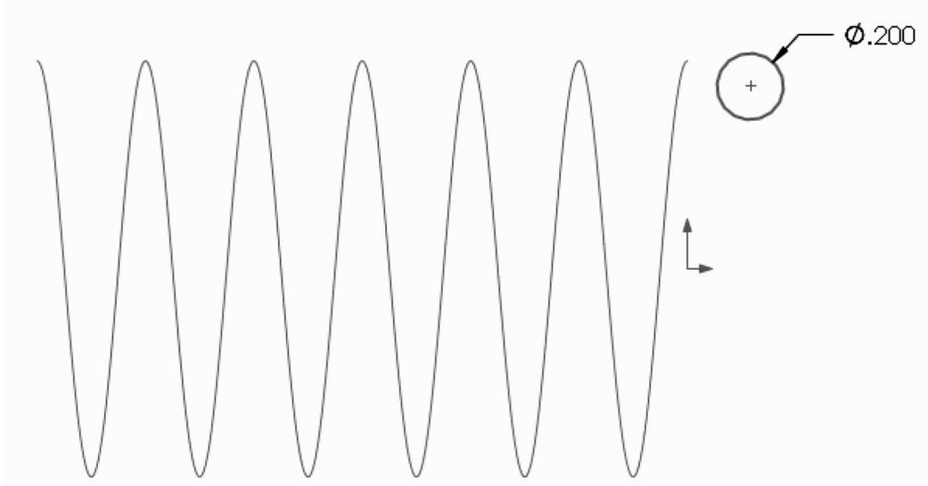
... and add a **“Pierce”** geometric relation between the center of the circle and the helix. This way the path will start at the beginning of the helix. This relation will make the sketch fully defined. Exit the Sketch when done.
