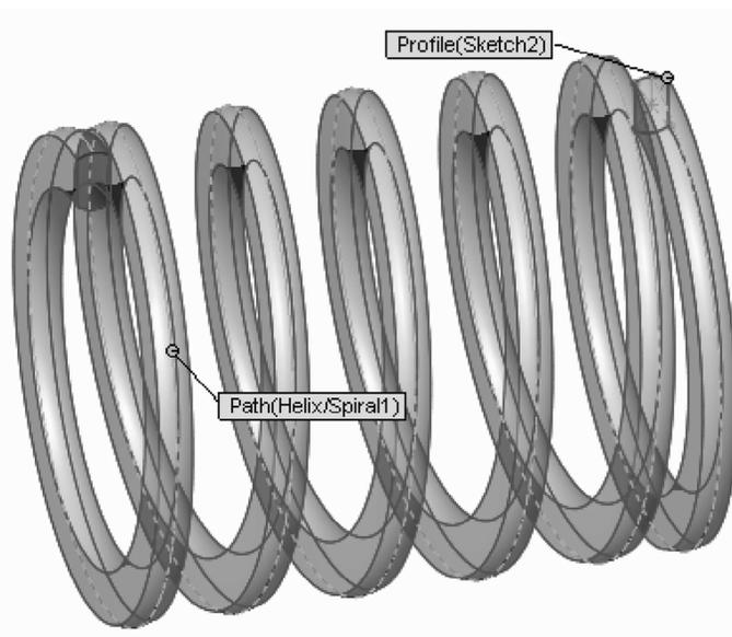
**170.** – To finish we'll make a cut to the sides to make the ends flat. Change to a Right view and add a sketch in the Right Plane. Draw a single line starting at the midpoint of the edge indicated, and down long enough to cross the part.
