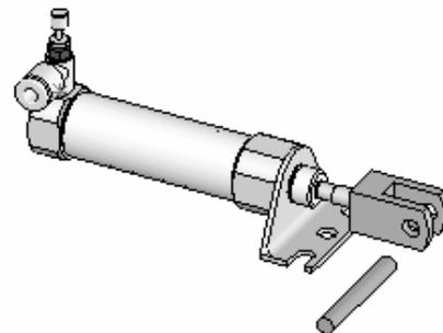
Insert a Concentric Mate between the RodClevis and the Axle. A Concentric Mate forces two cylindrical faces to become concentric. The faces can move along the common axis, but cannot be moved away from this axis.
