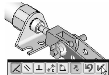
54. Perform the **same procedure** above to insert the second Shaft-Collar on the right side of the Flatbar.
