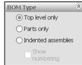
33. Click **OK**
