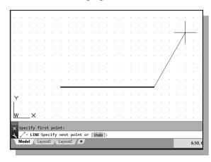
4. Next, create a vertical line by using the *relative polar coordinates entry method*, relative to the last point we specified:
