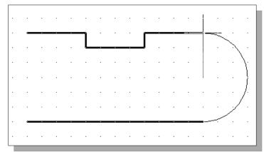
5. Move the cursor to the right endpoint of the top horizontal line as shown. Pick this point as the endpoint of the new arc.
