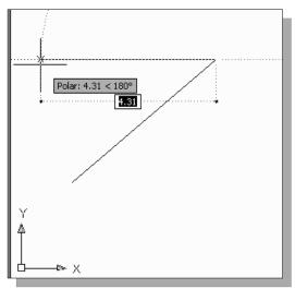
5. Move the cursor to the left of *point 2* and create a horizontal line about the same length as the first line on the screen.
