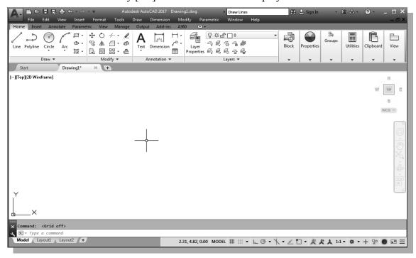
• Note that function key [F7] is a quick key, which can be used to quickly toggle on/off the grid display. Also, note the *command prompt area* can be positioned to dock below the drawing area or float inside the drawing area as shown.
