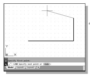
5. Next, we will use the direct input method. First, move the cursor directly to the left of the last endpoint of the line segments.
