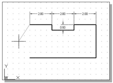
7. On your own, repeat the above steps and create the four additional line segments, using the dimensions as shown.
