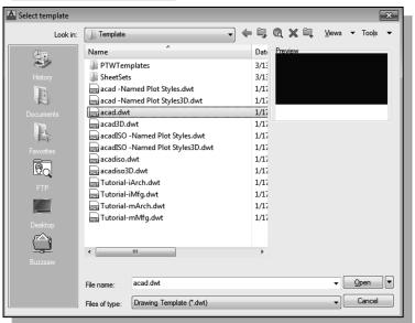
The dwt file type is the AutoCAD template file format. An AutoCAD template file contains predefined settings to reduce the amount of tedious repetitions.
