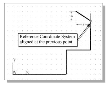
13. Using the *relative rectangular* coordinates entry method to create the next line, we can imagine a reference coordinate system aligned at the previous point.
