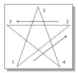
6. Repeat the above steps and complete the freehand sketch by adding three more lines (from *point 3* to *point 4*, *point 4* to *point 5*, and then connect to *point 5* back to *point 1*).
