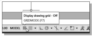
2. Move the cursor inside the graphics window, and estimate the distance in between the grid lines by watching the coordinates displayed at the bottom of the screen.
