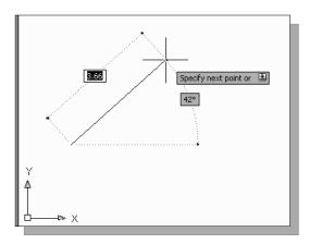
4. We will start at a location about one-third from the bottom of the graphics window. Left-click once to position the starting point of our first line. This will be *point 1* of our sketch. Next, move the cursor upward and toward the right side of *point 1*. Notice the rubber-band line that follows the graphics cursor in the graphics window. Left-click again (*point 2*) and we have created the first line of our sketch.
