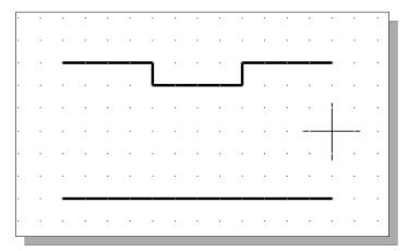
3. Move the cursor to the middle of the two horizontal lines and align the cursor to the two endpoints as shown. Click once with the **right-mouse-button** to select the location as the center point of the new arc.
