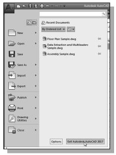
❖ To exit AutoCAD 2017, select Exit AutoCAD in the Menu Bar or type QUIT at the command prompt. Note the command can also be activated with the quick-key combination of [Ctrl]+[Q].
