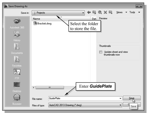
3. Click **Save** in the *Save Drawing As* dialog box to accept the selections and save the file. Note the default file type is DWG, which is the standard AutoCAD drawing format.
