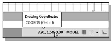
Note that the *coordinate display area* can also be used as a toggle switch; each left-mouse-click will toggle the coordinate display *on* or *off*.
