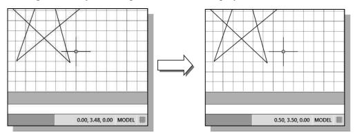
➤ The *GRID* option creates a pattern of lines that extends over an area on the screen. Using the grid is similar to placing a sheet of grid paper under a drawing. The grid helps you align objects and visualize the distance between them. The grid is not displayed in the plotted drawing. The default grid spacing, which means the distance in between two lines on the screen, is 0.5 inches. We can see that the sketched horizontal line in the sketch is about 4 inches long.
