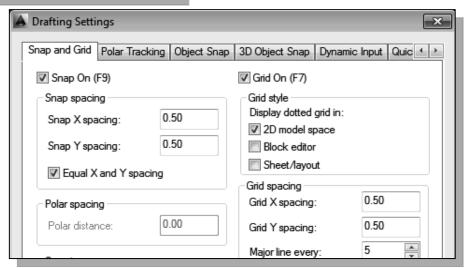
➤ On your own, exit the *Drafting Settings dialog box* and reset the status buttons so that only *GRID DISPLAY* and *SNAP MODE* are turned *ON* as shown.
