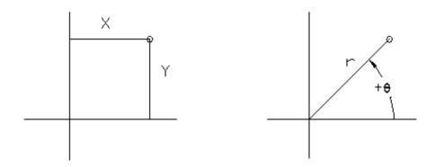
For planar geometry, the polar coordinate system is very useful for certain applications. In the polar coordinate system, points are defined in terms of a radial distance, r, from the origin and an angle  $\theta$  between the direction of r and the positive X axis. The default system for measuring angles in **AutoCAD 2017** defines positive angular values as counter-clockwise from the positive X-axis.
