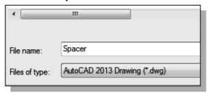
3. Click **Save** in the *Save Drawing As* dialog box to accept the selections and save the file. Note the default file type is DWG, which is the standard AutoCAD drawing format.
