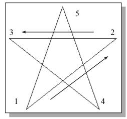
We will create a freehand sketch of a fivepoint star using the Line command. Do not be overly concerned with the actual size or accuracy of your freehand sketch. This exercise is to give you a feel for the AutoCAD 2017 user interface.
