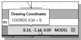
10. On your own, left-click on the coordinates display area to observe the switching of the coordinate display; set the display back to using the world coordinate system.
