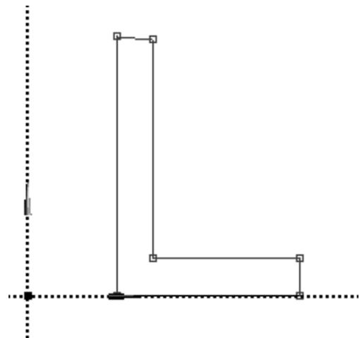
Use **constraint** options **horizontal** to make the top edge horizontal and **equal length** to make sure that the vertical and horizontal legs of the L are of the same thickness.
