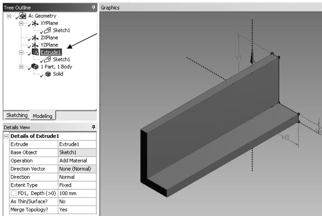
**Figure 1-17** Select the extrusion.
