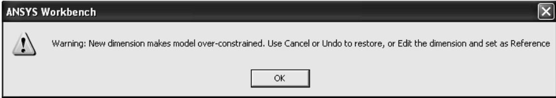
**Figure 1-28** Over-constraint message.
