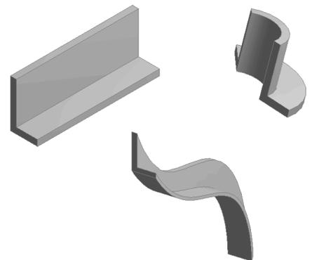
**Figure 1-1** Extruding, revolving, sweeping an L-shaped section.
