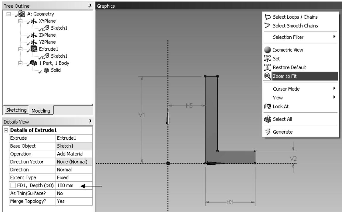
Figure 1-14 Extrusion.
