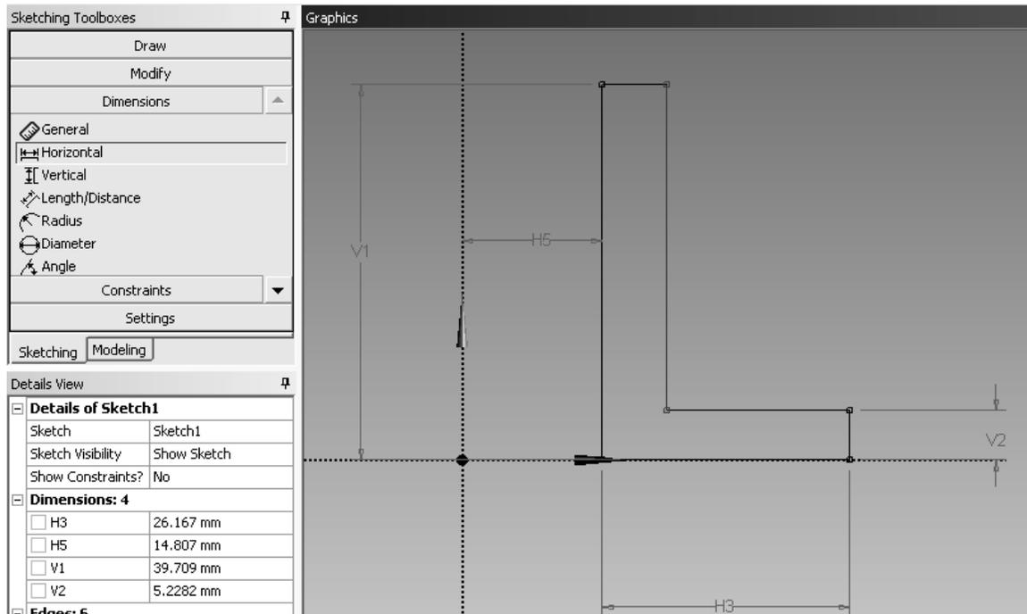
**Figure 1-11** L-section sketch with all dimensions.
