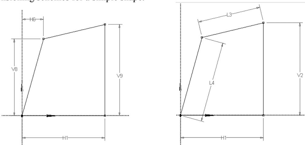
**Figure 1-27** Two different dimensioning schemes.
