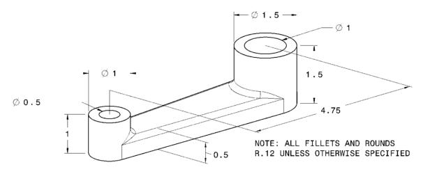
**P1-40)** Use a CAD package to create an orthographic projection of the following object. Draw the three standard views. Print using appropriate pen widths and insert a title block.
