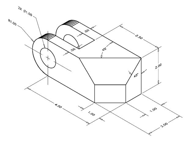
**P1-42)** Use a CAD package to create an orthographic projection of the following object. Draw the three standard views. Print using appropriate pen widths and insert a title block.
