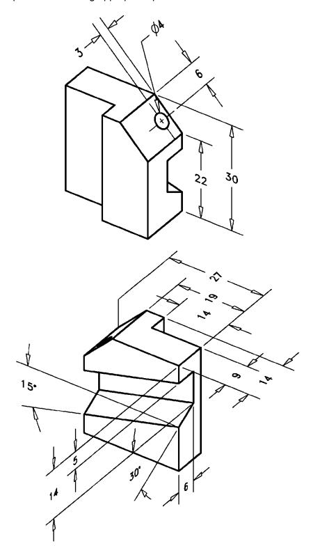
**P1-53)** Use a CAD package to create an orthographic projection of the following object. Draw an auxiliary view that shows the angled feature true shape. Use partial views where appropriate. Print using appropriate pen widths and insert a title block.
