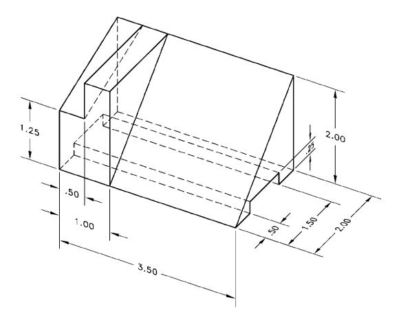
**P1-36)** Use a CAD package to create an orthographic projection of the following object. Draw the three standard views. Print using appropriate pen widths and insert a title block.
