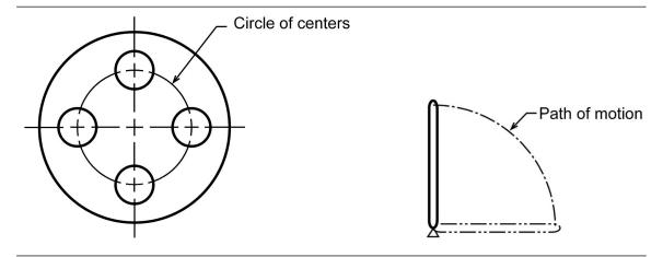
Figure 1-8: Center line uses
