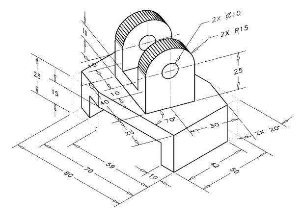
**P1-52)** Use a CAD package to create an orthographic projection of the following object. Draw two auxiliary views that show the angled features true shape. Use partial views where appropriate. Print using appropriate pen widths and insert a title block.
