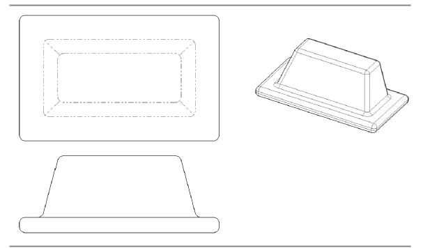
Figure 1-14: Phantom lines used to indicated a change in surface direction
