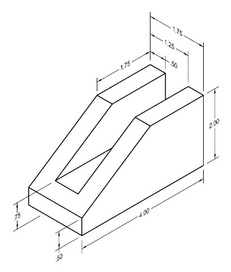
**P1-33)** Use a CAD package to create an orthographic projection of the following object. Draw the three standard views. Print using appropriate pen widths and insert a title block.
