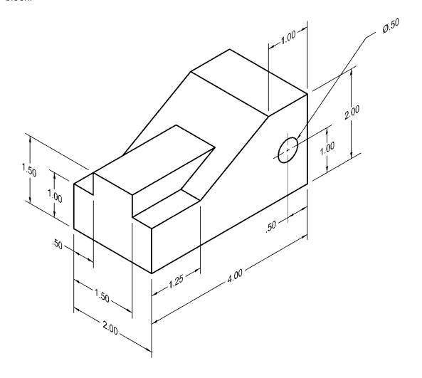
**P1-50)** Use a CAD package to create an orthographic projection of the following object. Draw an auxiliary view that shows the angled surface true shape. Use partial views where appropriate. Print using appropriate pen widths and insert a title block.
