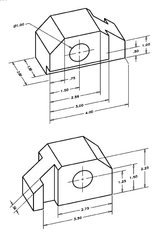
**P1-45)** Use a CAD package to create an orthographic projection of the following object. Draw the three standard views. Print using appropriate pen widths and insert a title block.
