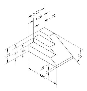
**P1-32)** Use a CAD package to create an orthographic projection of the following object. Draw the three standard views. Print using appropriate pen widths and insert a title block.
