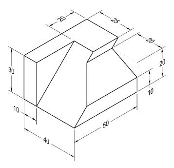
**P1-35)** Use a CAD package to create an orthographic projection of the following object. Draw the three standard views. Print using appropriate pen widths and insert a title block.
