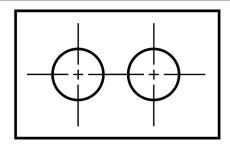
Figure 1-11: Connecting center lines.
