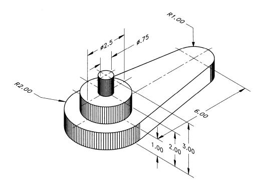
**P1-39)** Use a CAD package to create an orthographic projection of the following object. Draw the three standard views. Print using appropriate pen widths and insert a title block.
