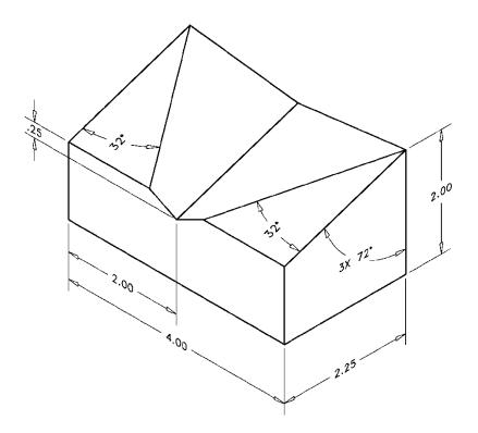
**P1-38)** Use a CAD package to create an orthographic projection of the following object. Draw the three standard views. Print using appropriate pen widths and insert a title block.
