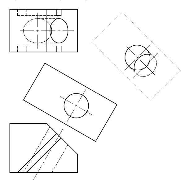
**P1-30)** Use a CAD package to create an orthographic projection of the following object. Draw the three standard views. Print using appropriate pen widths and insert a title block.
