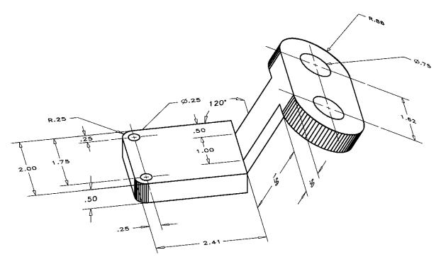
**P1-55)** Use a CAD package to create an orthographic projection of the following object. Draw an auxiliary view that shows the angled surface true shape. Use partial views where appropriate. Print using appropriate pen widths and insert a title block.
