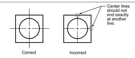
Figure 1-10: Terminating center lines.
