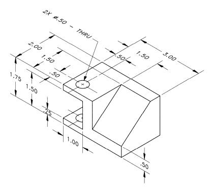
**P1-47)** Use a CAD package to create an orthographic projection of the following object. Draw the three standard views. Print using appropriate pen widths and insert a title block.
