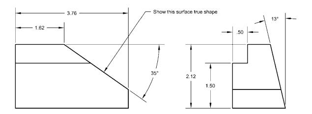
**P1-56)** Use a CAD package to create an orthographic projection of the following object. Draw an auxiliary view that shows the angled surface true shape. Use partial views where appropriate. Print using appropriate pen widths and insert a title block.
