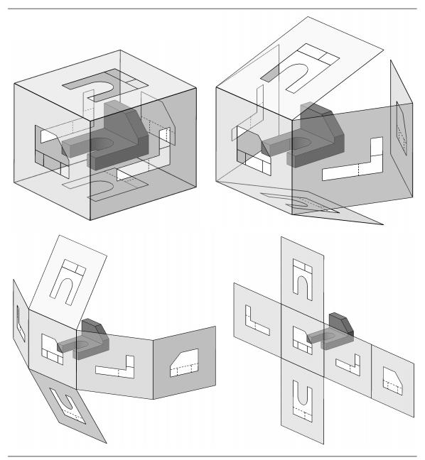
Figure 1-4: Glass box being unfolded.
