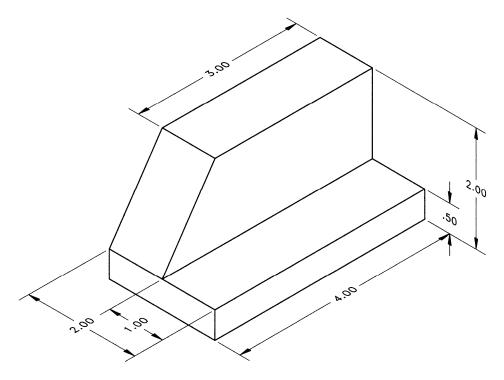
**P1-31)** Use a CAD package to create an orthographic projection of the following object. Draw the three standard views. Print using appropriate pen widths and insert a title block.
