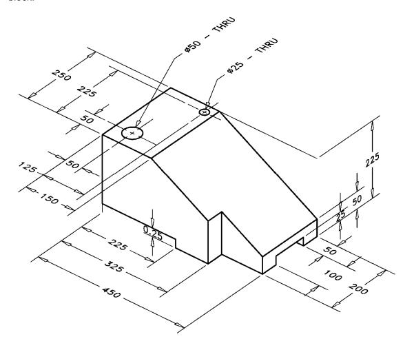
**P1-49)** Use a CAD package to create an orthographic projection of the following object. Draw the three standard views. Print using appropriate pen widths and insert a title block.
