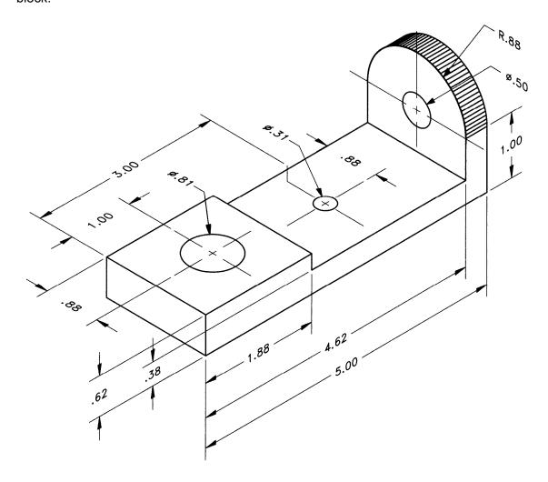
**P1-41)** Use a CAD package to create an orthographic projection of the following object. Draw the three standard views. Print using appropriate pen widths and insert a title block.
