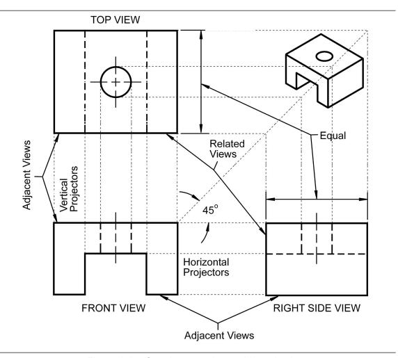
Figure 1-17: Creating an orthographic projection
