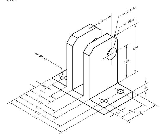
**P1-44)** Use a CAD package to create an orthographic projection of the following object. Draw the three standard views. Print using appropriate pen widths and insert a title block.
