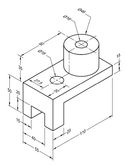
**P1-43)** Use a CAD package to create an orthographic projection of the following object. Draw the three standard views. Print using appropriate pen widths and insert a title block.
