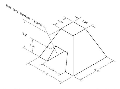
**P1-37)** Use a CAD package to create an orthographic projection of the following object. Draw the three standard views. Print using appropriate pen widths and insert a title block.
