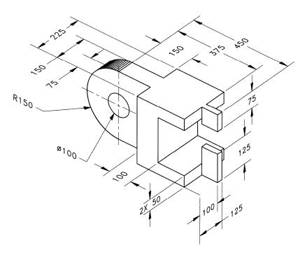
**P1-48)** Use a CAD package to create an orthographic projection of the following object. Draw the three standard views. Print using appropriate pen widths and insert a title block.
