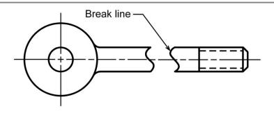
Figure 1-15: Using break lines.
