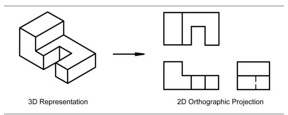
Figure 1-1: Orthographic projection.
