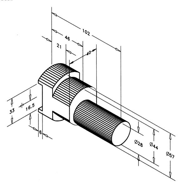
**P1-46)** Use a CAD package to create an orthographic projection of the following object. Draw the three standard views. Print using appropriate pen widths and insert a title block.
