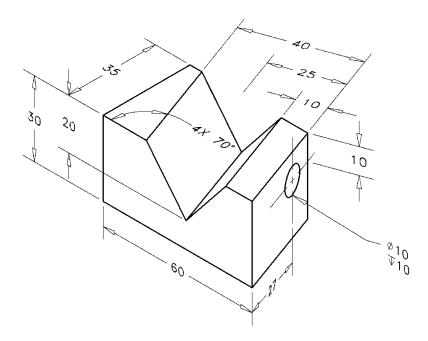
**P1-54)** Use a CAD package to create an orthographic projection of the following object. Draw an auxiliary view that shows the angled surface true shape. Use partial views where appropriate. Print using appropriate pen widths and insert a title block.
