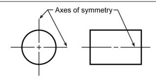
Figure 1-7: Axes of symmetry
