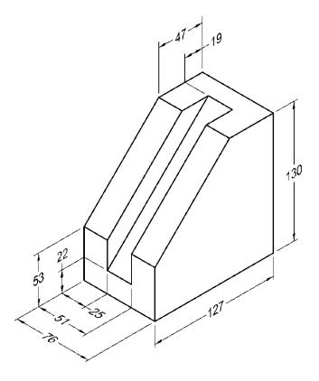
**P1-34)** Use a CAD package to create an orthographic projection of the following object. Draw the three standard views. Print using appropriate pen widths and insert a title block.
