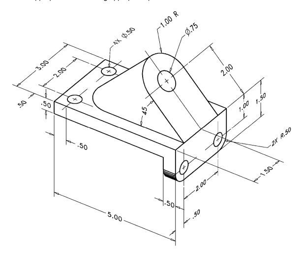
**P1-51)** Use a CAD package to create an orthographic projection of the following object. Draw an auxiliary view that shows the angled surface true shape. Use partial views where appropriate. Print using appropriate pen widths and insert a title block.
