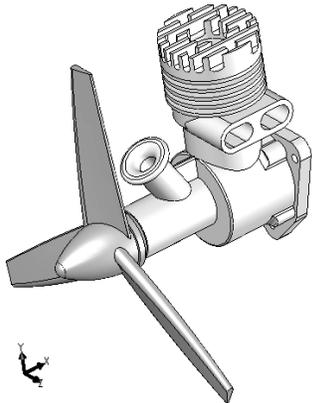
Figure 1-1 A Single Piston Engine (Unexploded View)
