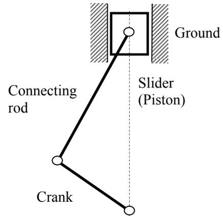
Figure 1-5 Schematic View of the Engine Motion Model
