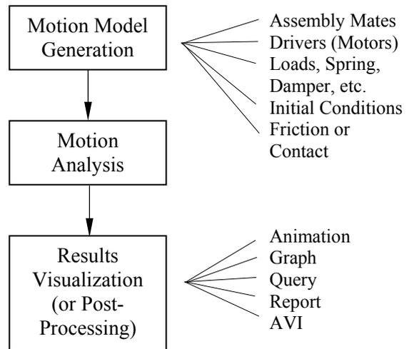
Figure 1-8 General Process of Using *SolidWorks Motion*
