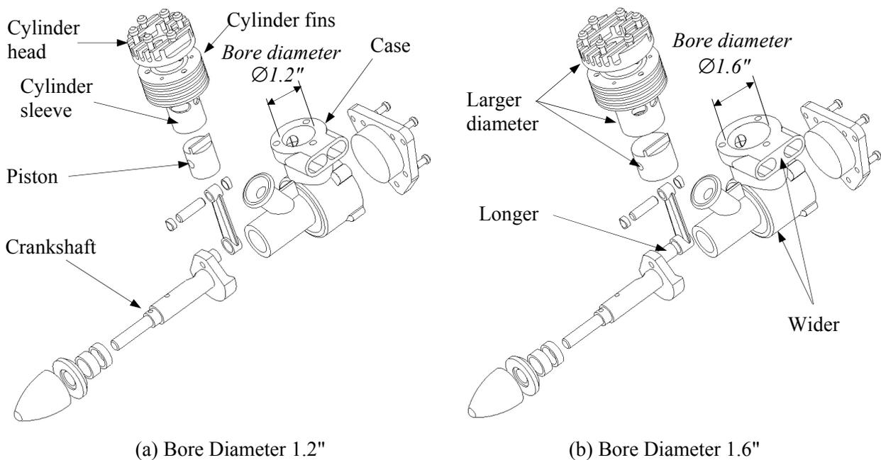
Figure 1-3 A Single-Piston Engine – Exploded View
