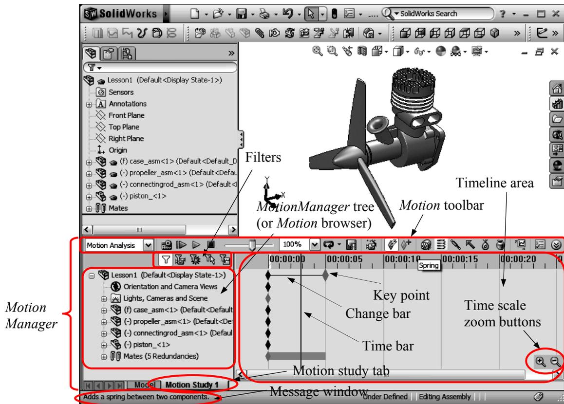
Figure 1-9 User Interface of *SolidWorks Motion* – *MotionManager*
