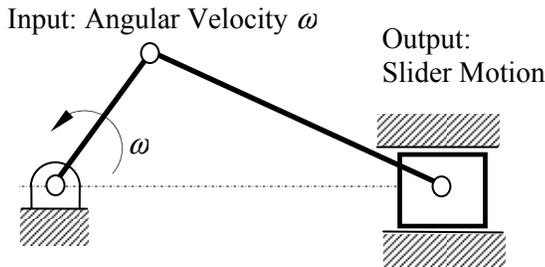
Figure 1-14 Kinematic Analysis
