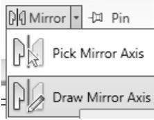
24. Select the center of the door as the start point of the mirror axis.
