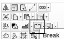
Locate the **Break** tool located on the Modify panel of the Home ribbon.
