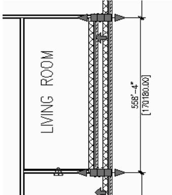
21. Locate the **CMU-190 Rigid-038 Air-050 Brick-090** wall style on the tool palette.
