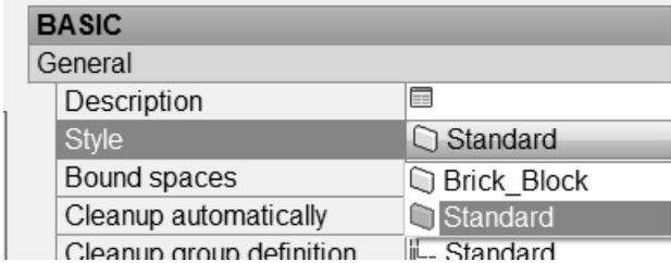
In the Properties dialog, check under the Style drop-down list. Only the Brick\_Block and Standard styles are available. *These are the wall styles that are loaded in the template.*
