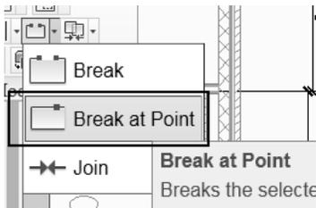
Select the **Break at Point** tool on the Break tool drop-down list to split the wall into two sections.
