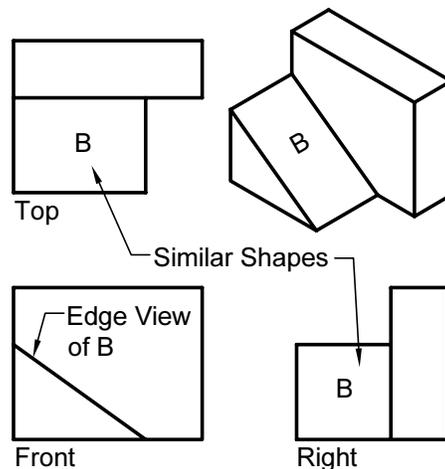
Figure MVD 12: Inclined plane “B” is in edge view in the front view and similar though foreshortened shapes in the top and right views
