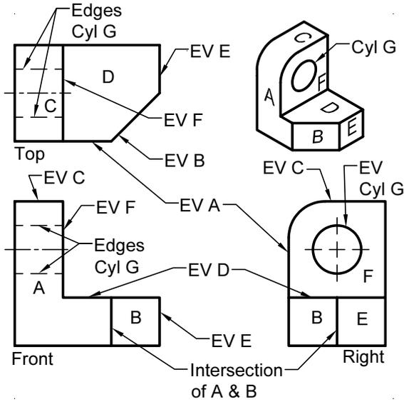
Figure MVD 15: Lines formed by the intersection of planes, EV of planes, and edges of arcs or cylinders
