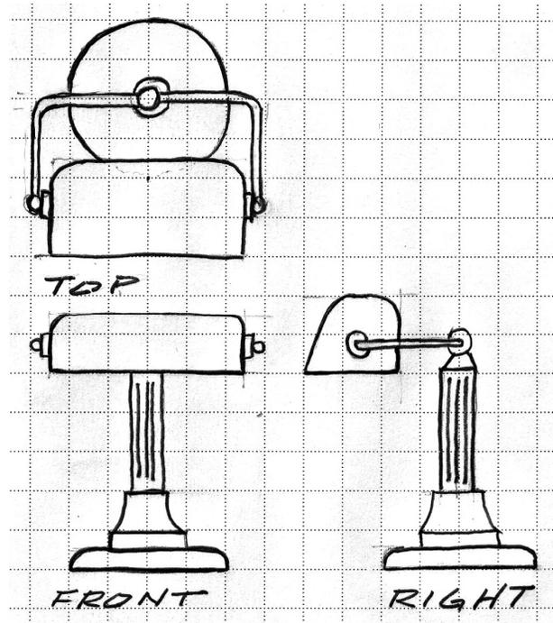
Figure MVD 1: Sketch showing the front, top, and right views of a table lamp
