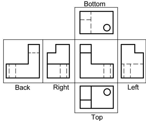
Figure MVD 20: Positioning of the six principle views in 1<sup>st</sup> angle projection
