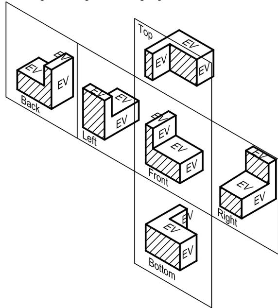
Figure MVD 9: The 3-D letter “L” with planes in or parallel to a principle plane shaded and planes perpendicular to a principle plane labeled EV
