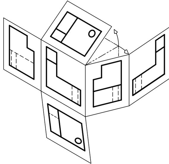
Figure MVD 5: All six planes of projection being unfolded about the front plane
