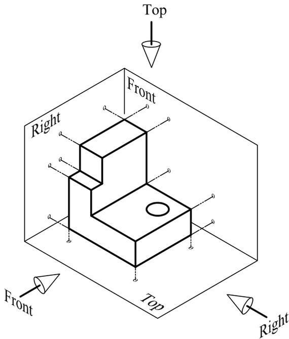
Figure MVD 19: the object is placed in front of the plastic planes in 1<sup>st</sup> angle projection
