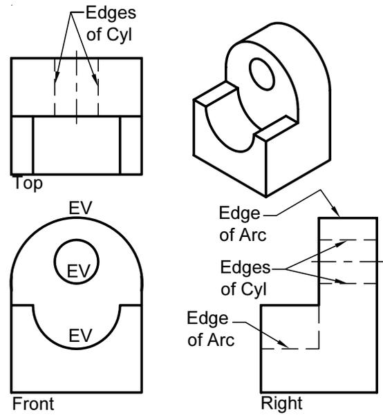
Figure MVD 14: Single curved surfaces display as edge views in the front view and as lines in the top and right views
