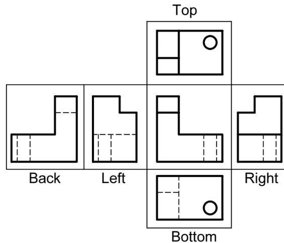
Figure MVD 6: All six sides of the plastic box unfolded into the 2-D plane of a piece of paper.
