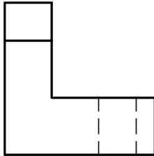
Figure MVD 4: Resulting front orthographic view as projected onto the front plane of projection
