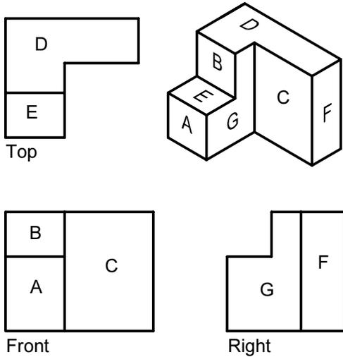
Figure MVD10: No way of telling which plane is closer
