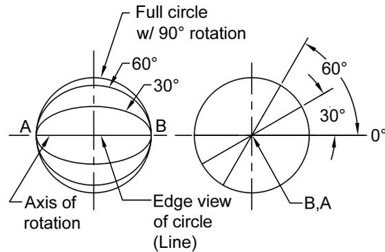
Figure MVD 18: The rotating circle starts as a line then forms two different ellipses and finally a full circle
