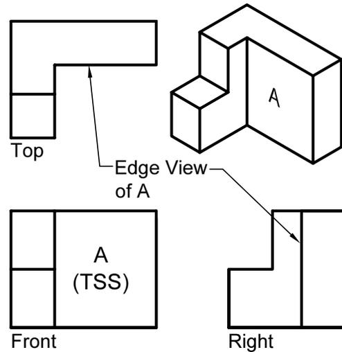
Figure MVD11: Normal plane “A” is true size and shape in the front view and is in edge view in the top and right views
