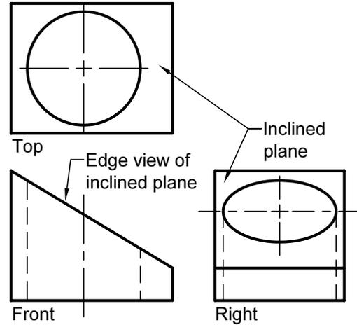
Figure MVD 17: A hole appears as an ellipse when in an inclined plane
