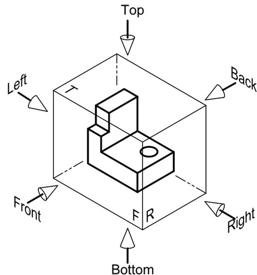
Figure MVD 2: Object encased in a clear plastic box with arrows locating the viewing position of the six principle orthographic views
