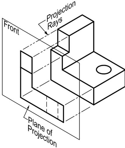
Figure MVD 3: Projection rays projecting the front view of the object onto the front plane of projection
