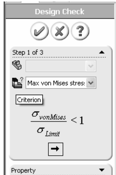
Figure 21 – First Design Check property manager. The comparison stress (criteria) is selected here.
