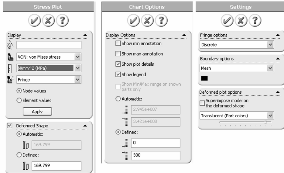
Figure 2-24: Stress Plot (invoked by Edit Definition...), Chart Options and Settings windows we use in this exercise to modify stress plot display
