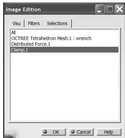
As the postprocessing proceeds and we generate different plots, they are recorded in the tree as shown. Each plot generated deactivates the previous one on the screen. By pointing to a desired plot in the tree and right clicking, you can activate the plot. Clearly any plot can be deleted from the tree in the usual way (right click, **Delete**).
