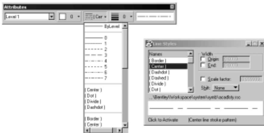
Figure 3-14. Selecting a custom line style from attributes toolbar and line style dialog.
