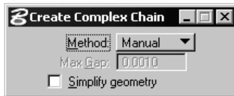
Figure 3-5. Create complex chain tool settings box.
