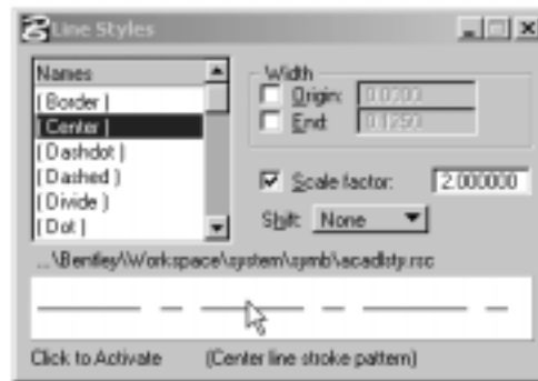
Figure 3-15. Activating modifiers for a custom line style.
