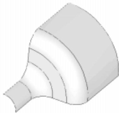
Figure 4 3D Shell quarter-model of transition between cylinders
