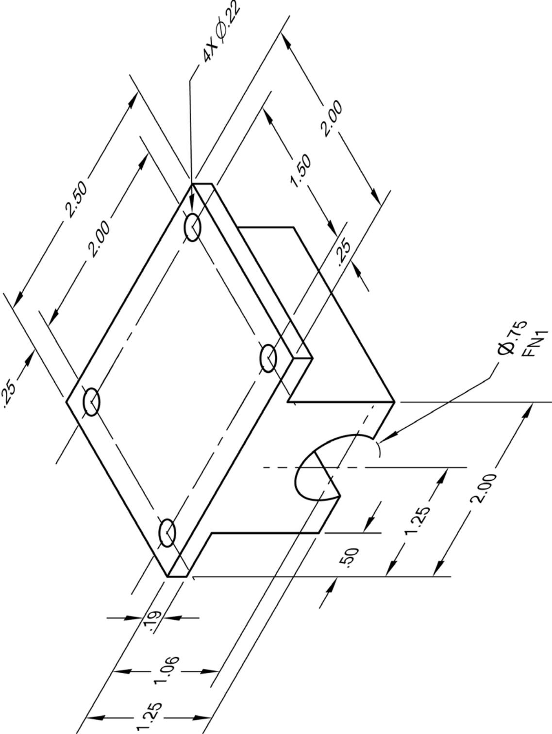
Part#5: Bearing If you are just studying the basics and have not covered tolerancing, ignore the RC4 and FN1 tolerances.
