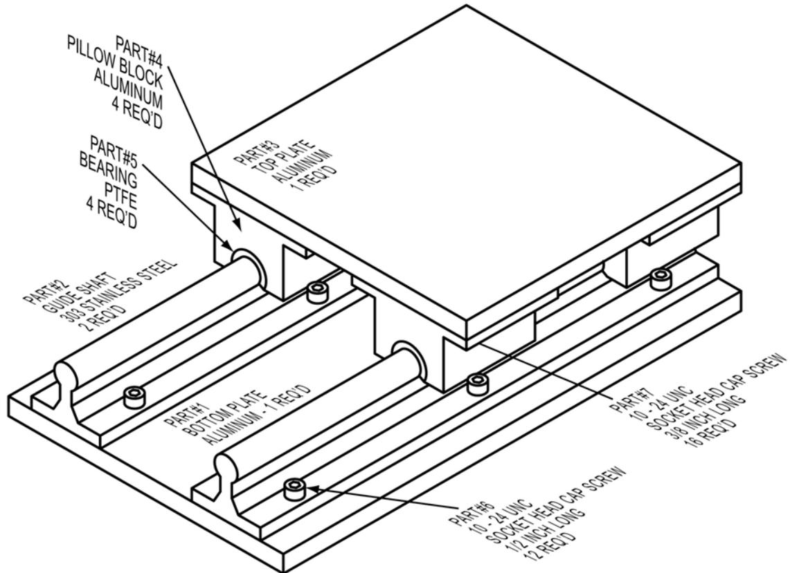
Part#2: Gui de Shaft If you are just studying the basics and have not covered tolerancing, ignore the RC4 tolerance. NOTE TO DRAFTER: This part is symmetric and all fillets are R.12.
